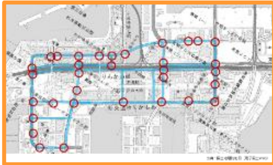
Installed V2I (760MHz) equipment at 33 intersections in Odaiba
