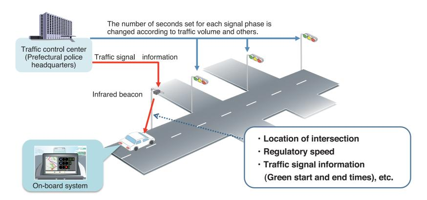
Infrastructure provides information to the vehicle's on-board unit, such as signal information of an intersection through which the vehicle is going to pass and the distance to the intersection. The on-board unit provides the above-mentioned four support via HMI based on the information obtained from the infrastructure and the information on its own vehicle.
