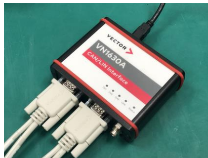
Fig2. Vector VN1630A + CANPiggy × 2 上記はCANoeで制御
