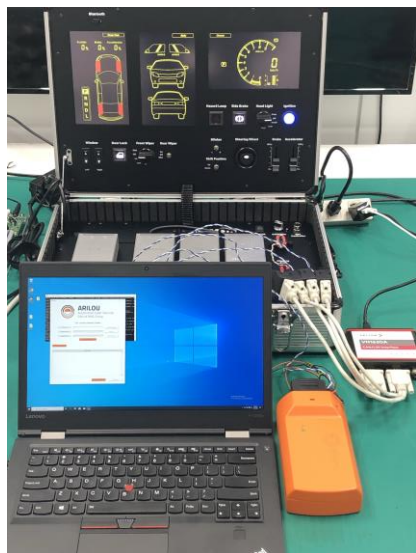
Fig2. Vector VN1630A + CANPiggy × 2 上記はCANoeで制御
