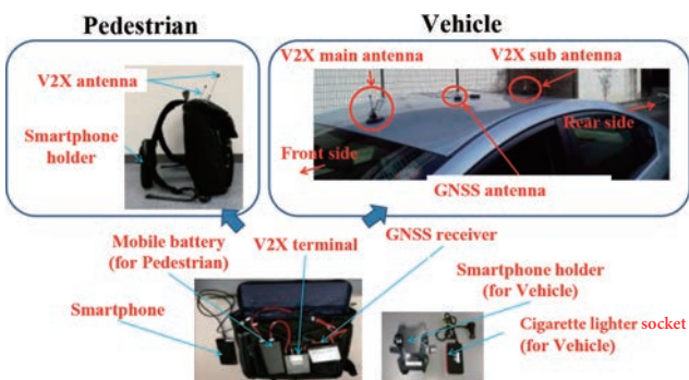
Fig.17. Exterior views of terminal prototypes
