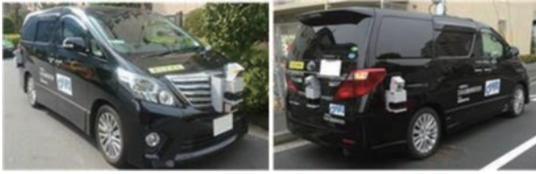
Fig. 1 Vehicle developed for collecting driving video data
